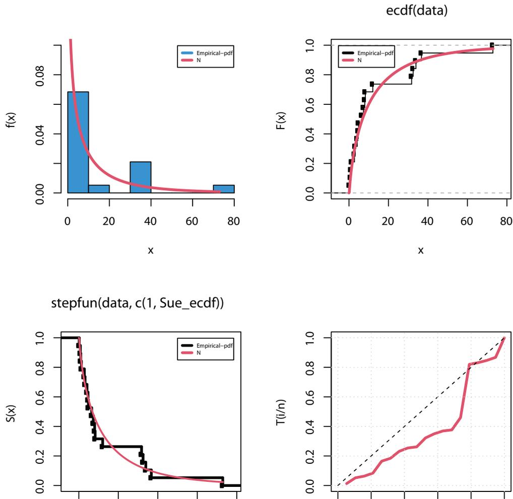
Figure 10: Density, cdf, survival, and TTT plots for the data on time to break down of an insulating fluid between electrodes at a voltage of 34 k.v. (minutes).
